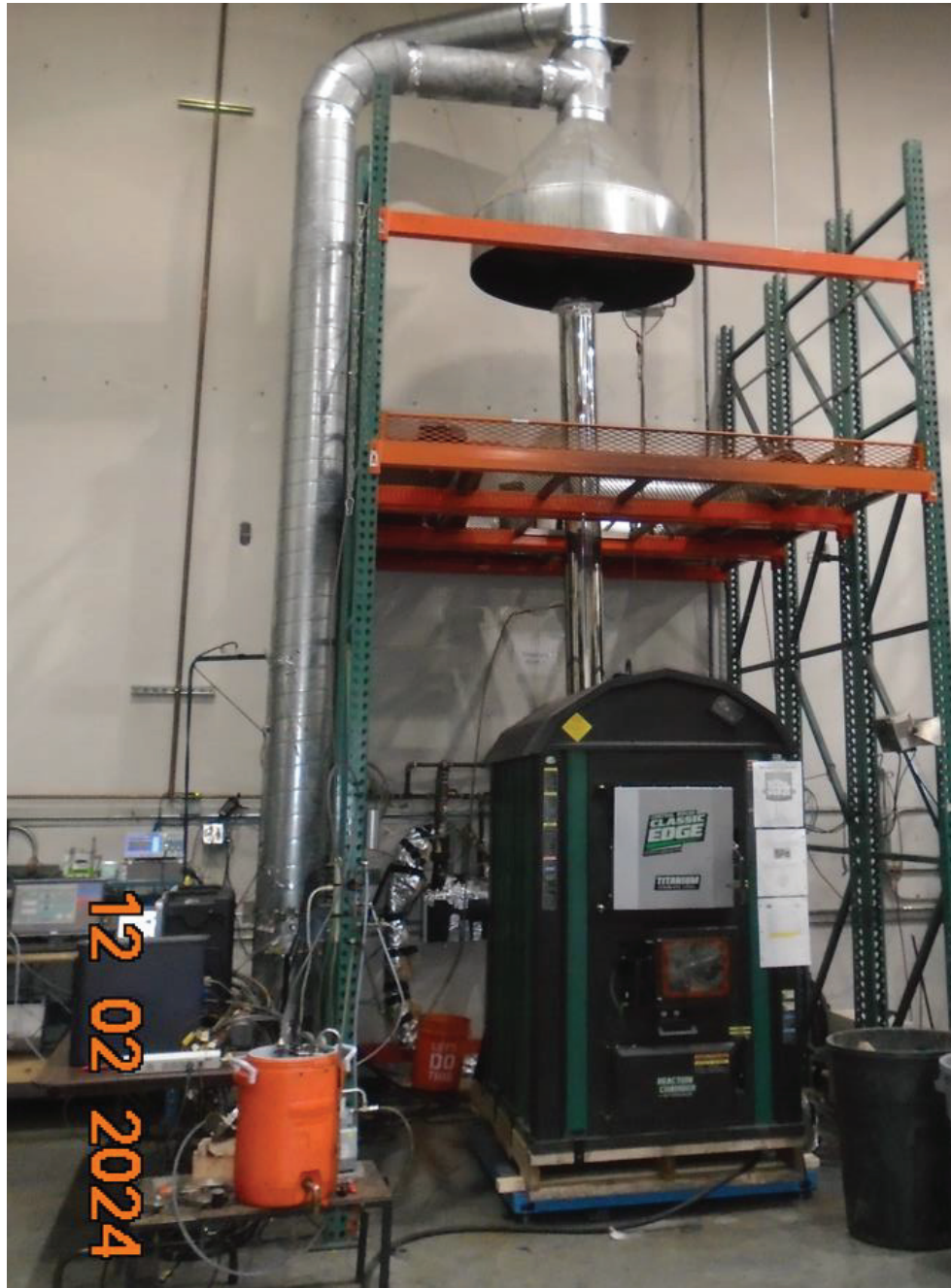
Figure 7 - Central Boiler Classic Edge 560.1 installed in test structure and general work area
