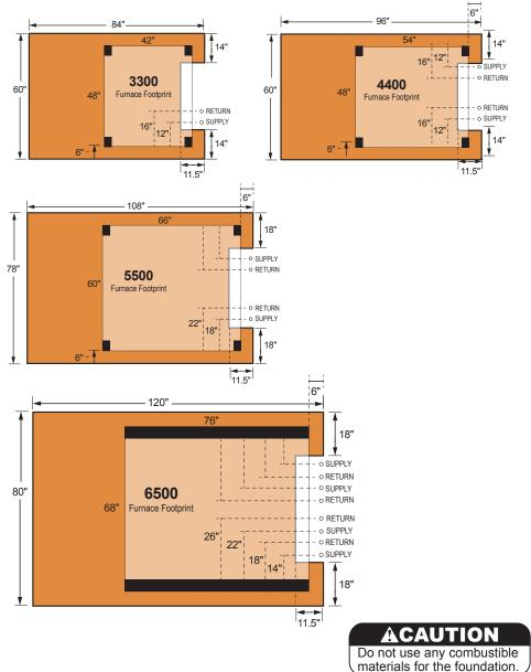
Outdoor furnace must be installed on a noncombustible surface or foundation that incorporates an enclosure that will prevent supply and return lines from possible exposure to sunlight, fire, or physical damage that may be caused by an occurrence outside the outdoor furnace enclosure. Foundation may consist of concrete, crushed rock, or patio blocks.
